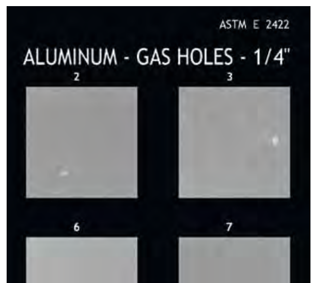
ASTM reference images for aluminum according to ASTM E2422
