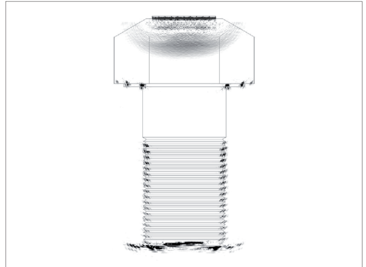
TFM-image of a screw by using a grey-scale, insonification from the top
