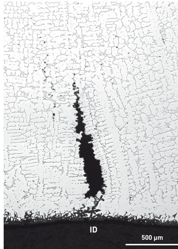
Figure 7: Higher magnification photomicrograph of creep fissure
