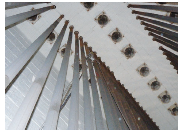
Reformer tube testing with LEO-Scan
