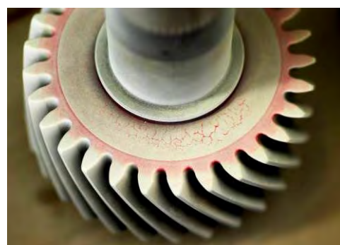
Defects indication effected by contrast penetrant system application
