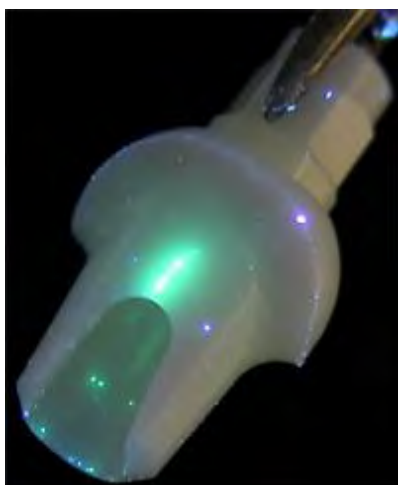
Defects indication effected by fluorescent penetrant system application
