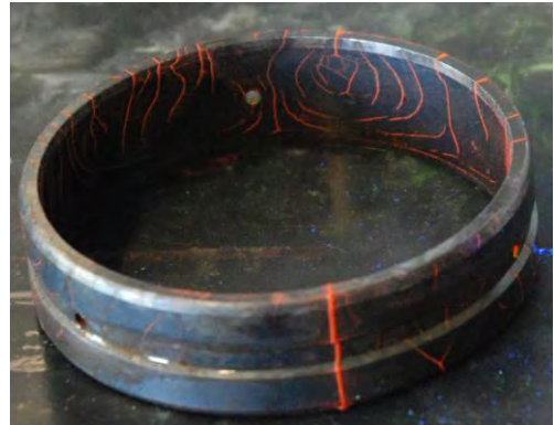
Defect indication after application of red water-suspended magnetic particles type MEF 515
