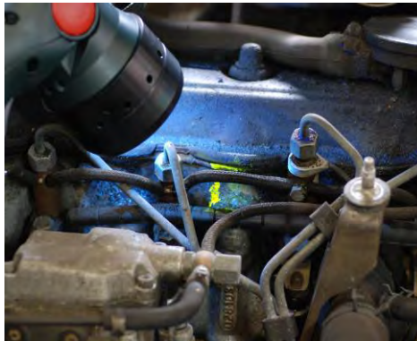
Leak detection in automobile engine by use of H 800 fluorescent concentrate
