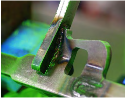
Defect indication after application of fluorescent water based magnetic particle suspension type LY 1500
