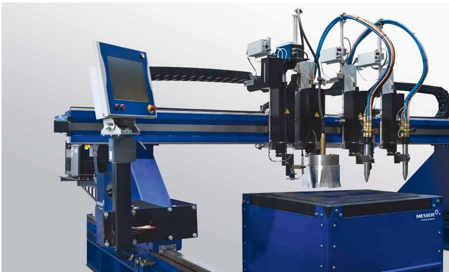
The user-friendly control Global Control speeds set-up and reduces errors and non-productive times.
