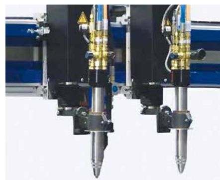
Multiple ALFA torches with quick nozzle change permit high productivity.
