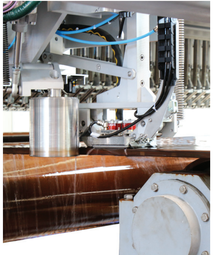
Edge inspection carriages
