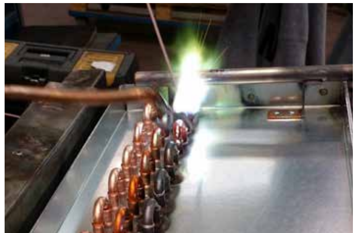
Standard technology with loss of phosphorus and sparking resulting in increased leakage.
