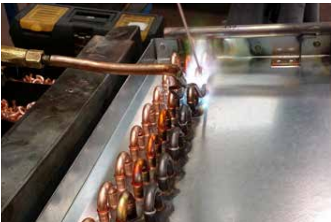
NanoPhos™ technology with no loss of phosphorus, not boiling or sparking of the alloy in the brazed joint. Result is 50% few leaks.
