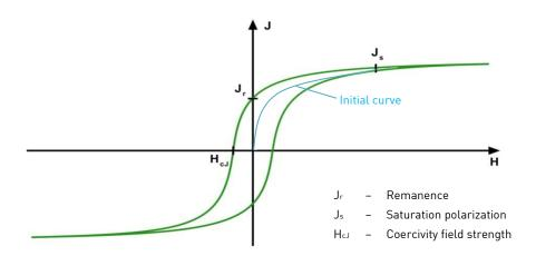
For magnetization into saturation polarization Js, a magnetization field of up to 200 kA/m is available. Additionally a pulse magnetization of 450 kA/m for hard magnetic specimen with HcJ more than 50 kA/m is available as an option.
